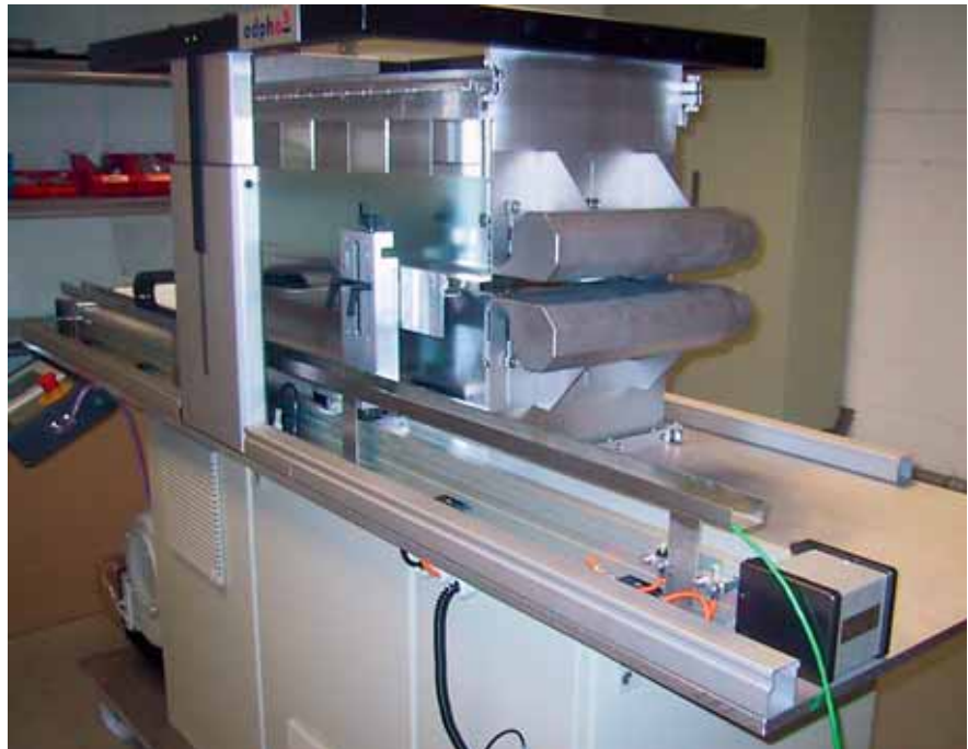
Figure 6, above: Section of a NIR ® -curing oven for the final coating/curing.
