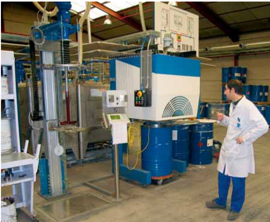
A fully-automated mixing unit, featuring online access to the Beckers support team, combines immediate on-site industrial mixing capability with full technical backup. Just-in-time paint!
